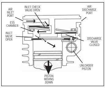
FIGURE 4 - OPERATIONAL-LOADED (INTAKE)
