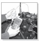
Testing the temperature at the discharge fitting.
