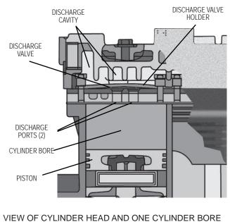
FIGURE 1 - DURAFLO 596™ AIR COMPRESSOR
