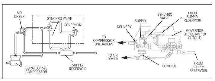
FIGURE 3 - DURAFLO 596™ AIR COMPRESSOR UNLOADER SYSTEM
