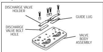
FIGURE 11 - DISCHARGE VALVE INSTALLATION
