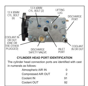
FIGURE 9 - TYPICAL DURAFLO 596™ AIR COMPRESSOR CYLINDER HEAD
