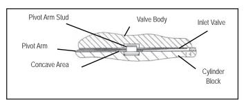
FIGURE 12 - SLIDING INLET VALVE INSTALLATION
