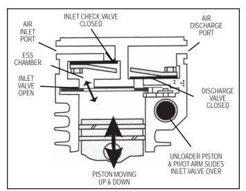
FIGURE 6 - OPERATIONAL-UNLOADED
