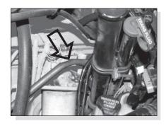
Damaged discharge line shown.
