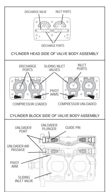
FIGURE 7 - UNLOADER MECHANISM
