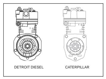
FIGURE 2 - TYPICAL COMPRESSOR DRIVE FLANGES
