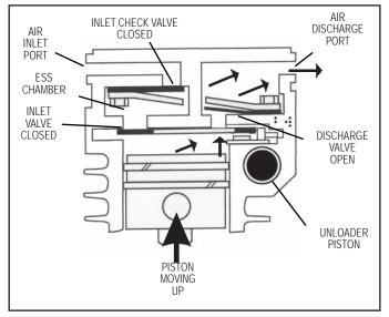
FIGURE 5 - OPERATIONAL-LOADED (COMPRESSION)
