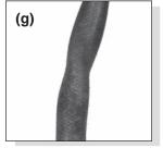
Partly collapsed inlet line shown.
