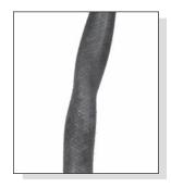
Partly collapsed inlet line shown.
