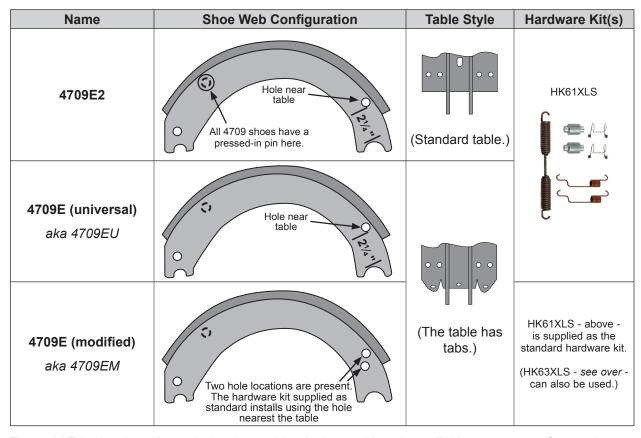
The 4709E brake shoe shown below is an older design and is only available as a remanufactured component.
