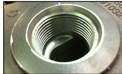
INLET PORT THREADS ARE IN GOOD CONDITION
