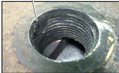
INLET PORT THREADS ARE DAMAGED
