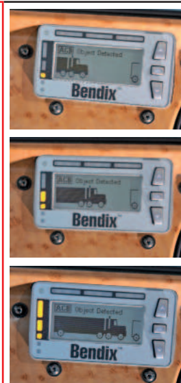
FIGURE 9 - DRIVER INTERFACE UNIT (DIU) SHOWING EXAMPLES OF FOLLOWING DISTANCE ALERTS WITH PROGRESSIVELY FASTER AUDIBLE ALERTS.
