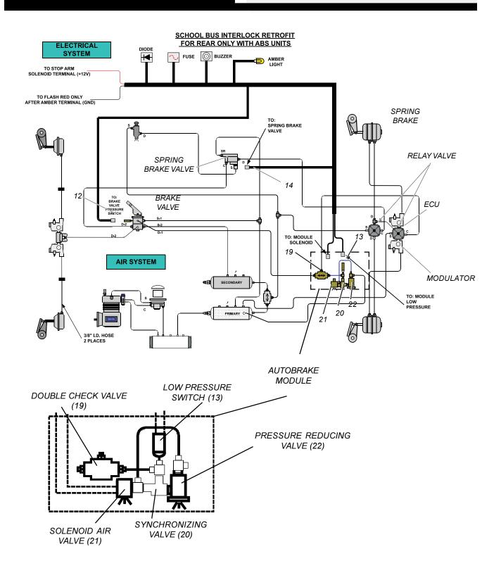
AutoBrake sequential kit part number 5008285 installed on a vehicle with antilock.
