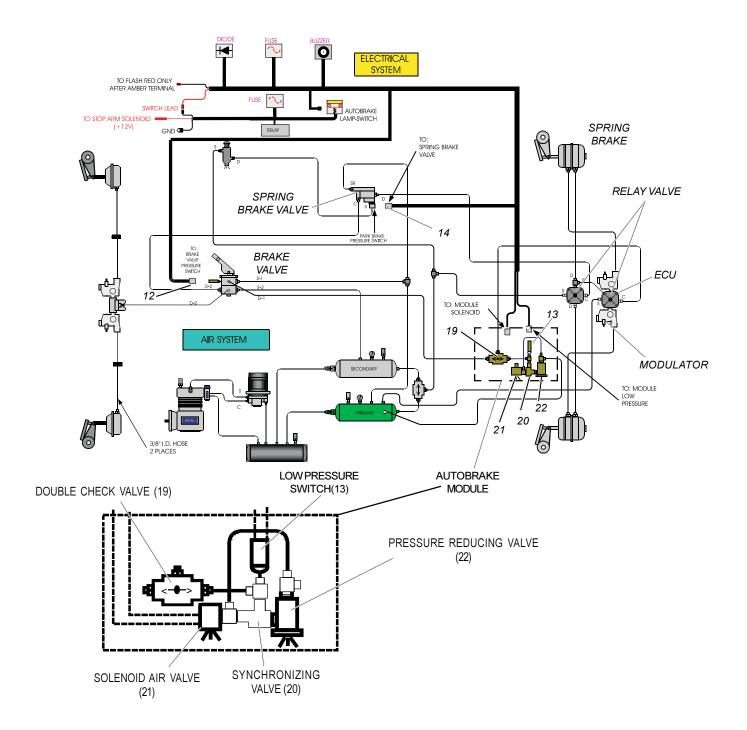
AutoBrake non-sequential kit part number 5011053 installed on a vehicle with antilock.
