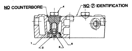
When service replacement of any of the following parts is required, all of the following parts must be removed and should not be reused in the old style cylinder head.
