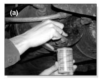
Drain <u>all</u> air tanks (reservoirs) into the Bendix<sup>®</sup> BASIC test cup. (Bendix kit P/N 5013711).
