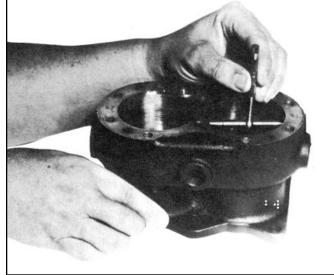
FIGURE 21 - MEASURING CYLINDER BORES
