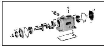
FIGURE 19 - CRANKCASE - TU-FLO<sup>®</sup> 400 & 500 AIR COMPRESSORS
