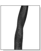
(h) Restricted air inlet (not enough air to compressor). 25 inches of water. ⇒ Check the engine air filter and service if Partlv usage indicator). collapsed inlet line Check shown.
