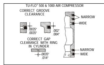
FIGURE 24 - PISTON RING POSITIONS - GAPS AND GROOVE CLEARANCE
