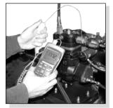
Testing the temperature at the discharge fitting.
