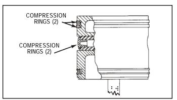
FIGURE 22 - TU-FLO® 400 AIR COMPRESSOR NEW STYLE
