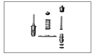
FIGURE 25 - UNLOADER MECHANISM
