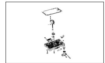
FIGURE 18 - BASE PLATE SELF-LUBRICATED TYPE COMPRESSOR
