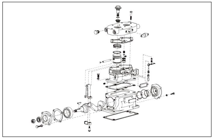
FIGURE 17 - TU-FLO® 400 AIR COMPRESSOR VERTICAL MOUNT - ENGINE LUBRICATED
