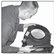
Inspect the engine air cleaner.
