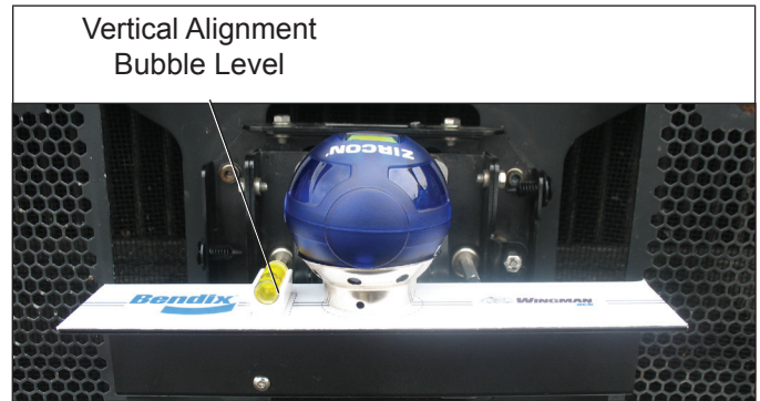
FIGURE 30 - VERTICAL ALIGNMENT BUBBLE LEVEL
