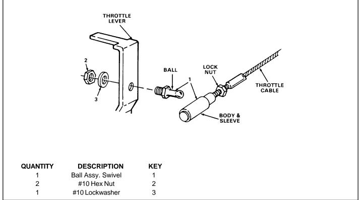
Figure 1 This kit consists of the parts listed above.
