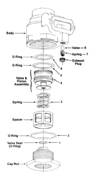
Figure 1 - Inlet Regulating Valve
