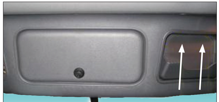
Figure 3 - Freightliner Vehicle Processor Location
