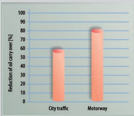
Reduction of oil carry over of a compressor with clutch in comparison with a standard compressor
