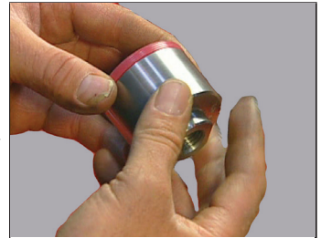
Figure 82 – Position the New Boot in the Sleeve Installation Tool (T07)
