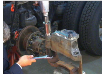
Figure 71 – Remove the Long Guide Pin
