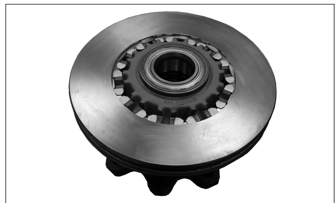
Figure 90 – Intermediate Elements (Spacers Installed)
