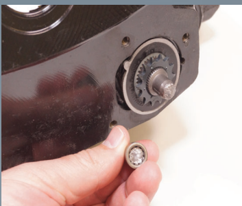
Failed adjuster / Requires caliper replacement
