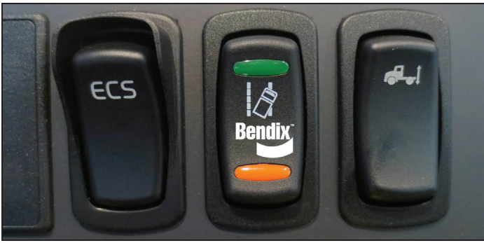
Figure 7 – Example Enable/Disable Switch Installation
