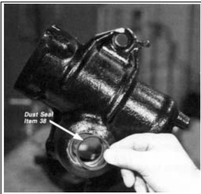
FIGURE 30 - REMOVING/INSTALLING HOUSING OUTPUT SHAFT DUST SEAL
