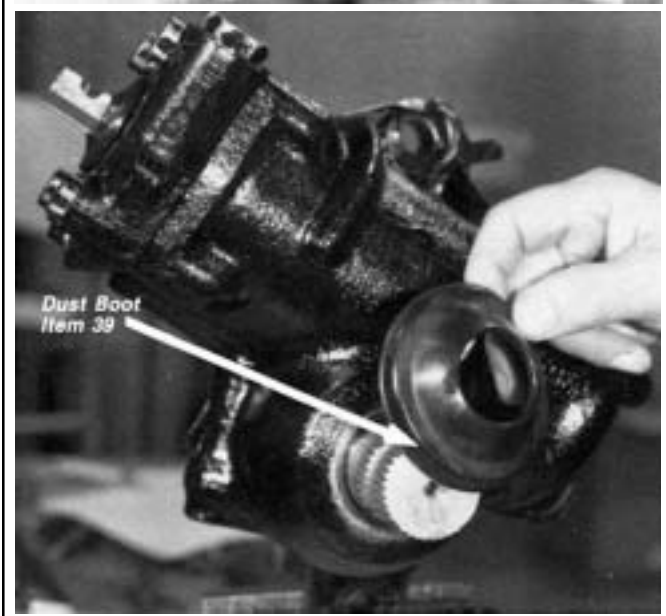
FIGURE 16 - REMOVING/INSTALLING PITMAN ARM & DUST BOOT
