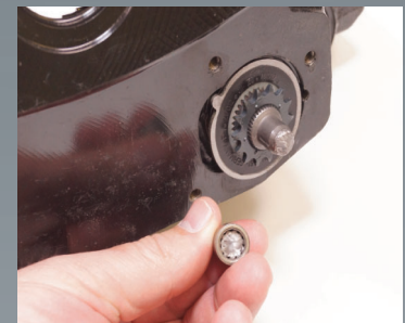
Failed adjuster / Requires caliper replacement
