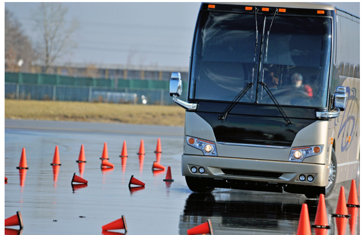
With the Bendix® ESP® activated, the vehicle repeats the course navigating the same maneuver safely. (Note: In production, the Bendix® ESP® system can not be turned off by the driver).
