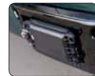
Bendix® FLR20™ Radar Sensor Mounted to the Vehicle Front
