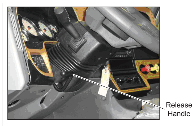
Figure 1 Tilt-Telescoping Steering Column Release Handle
