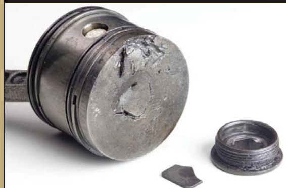
Poor quality replacement pieces
