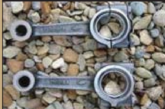
Poor bearing surfaces
