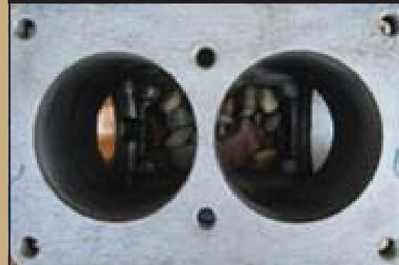
Poor machining & scratches
