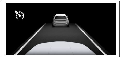
Figure 6b – ACB Canceled, AEB Detecting the Forward Vehicle
