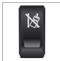
Figure 19 – LDW, HDW, and HDB Disable Switch
