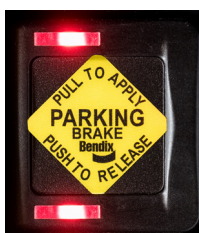
Dash Electronic Control Unit (DECU) Included with the Bendix® Intellipark® EPB System
