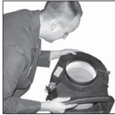
Inspect the engine air cleaner.
