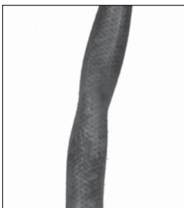
Partly collapsed inlet line shown.
