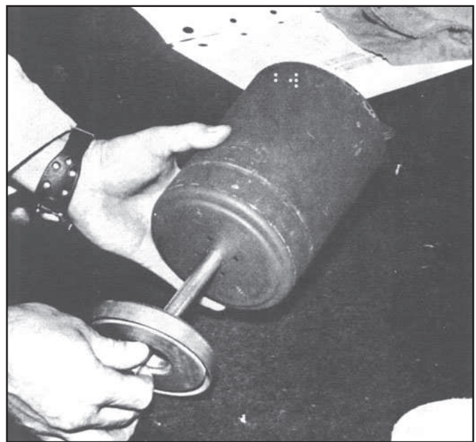
Figure 10 – Cartridge Bolt Installation
