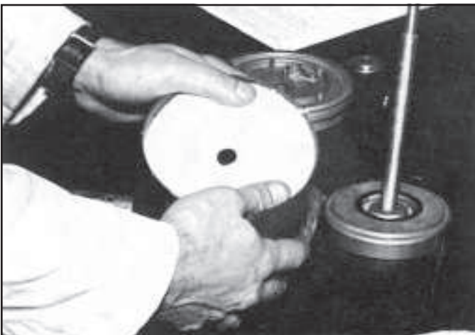
Figure 8 – Desiccant Cartridge Assembly
