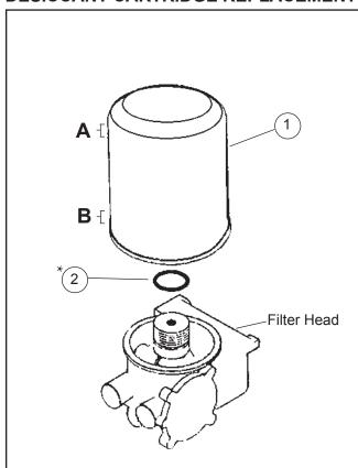
The desiccant cartridge replacement kit consists of the following:
