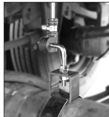
FIGURE 8 - THE VERTICAL LINKAGE ROD ATTACHES TO THE AXLE USING THE FINE-ADJUSTMENT LINKAGE.
