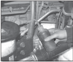
Testing for leaks with soap solution.
