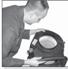
Inspect the engine air cleaner.
