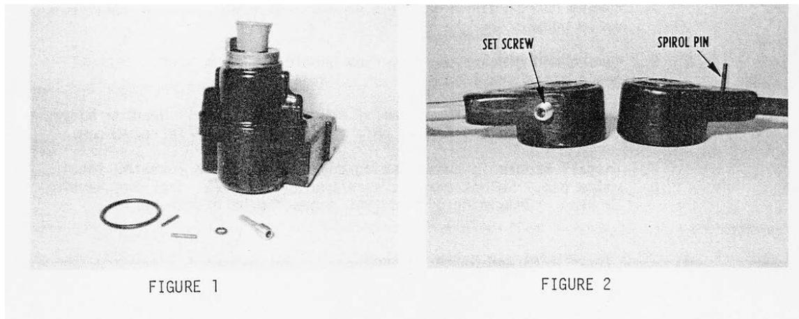
Included with all Remanufactured TC-2 Valves will be the necessary detail parts to accomplish head/handle changeover for all style valves. Unused parts may be discarded. Included with the valves will be the following parts. (See Figure 1)
