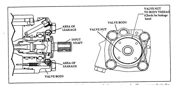
Leakage in this area can be visually noted without removal of any parts and will appear early in the service life of the power steering gear; generally under 5,000 miles. The intensity of leakage will vary from a barely detectable "weep" to as much as 10 drops per minute. The leakage described is from the oil return (low pressure) side of the power steering gear.
