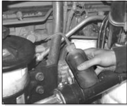
Testing for leaks with soap solution.
