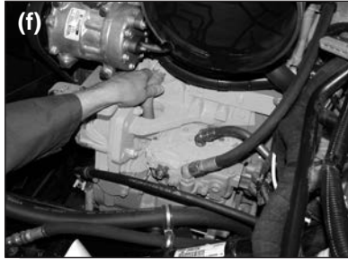
Inspecting the coolant hoses.
