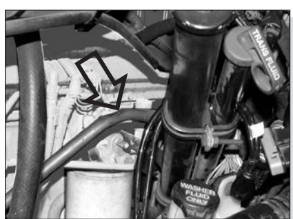
Damaged discharge line shown.
