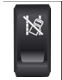
Figure 17 – LDW, HDW, and HDB Disable Switch
