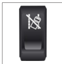
Figure 19 – LDW, HDW, and HDB Disable Switch
